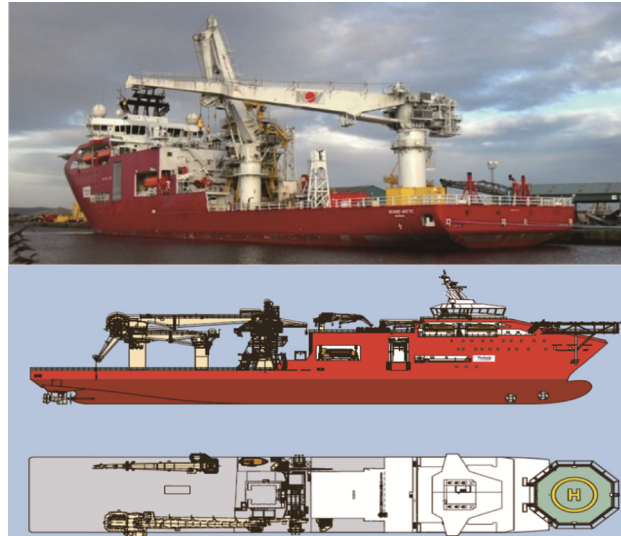
Fig. 9. The configuration and deck plan of Skandi Arctic (Kupen, 2009).
