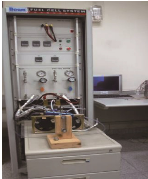
Fig. 6. Performance test equipment of PEMFC.
