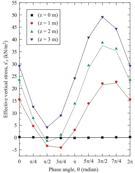
Fig. 5. Effective Vertical stress for loose sand seabed.
