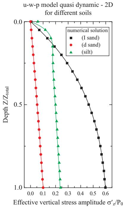
Fig. 4. Effective Vertical stress amplitude for different soils.
