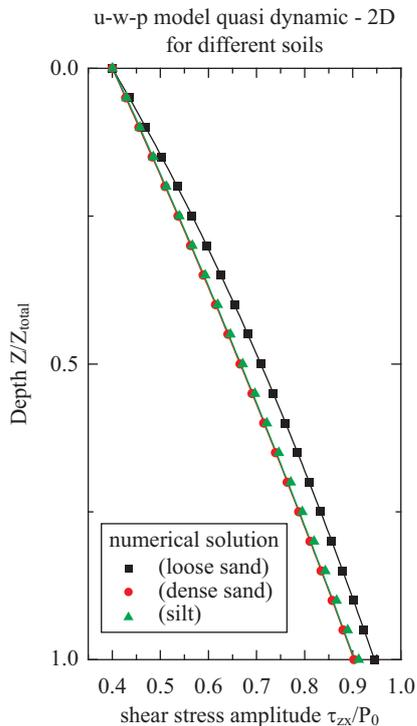
Fig. 6. Shear Stress variation for different seabed.
