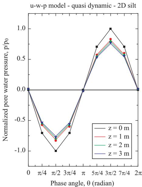
Fig. 2. Normalized Pore water pressure variation for silty seabed.
