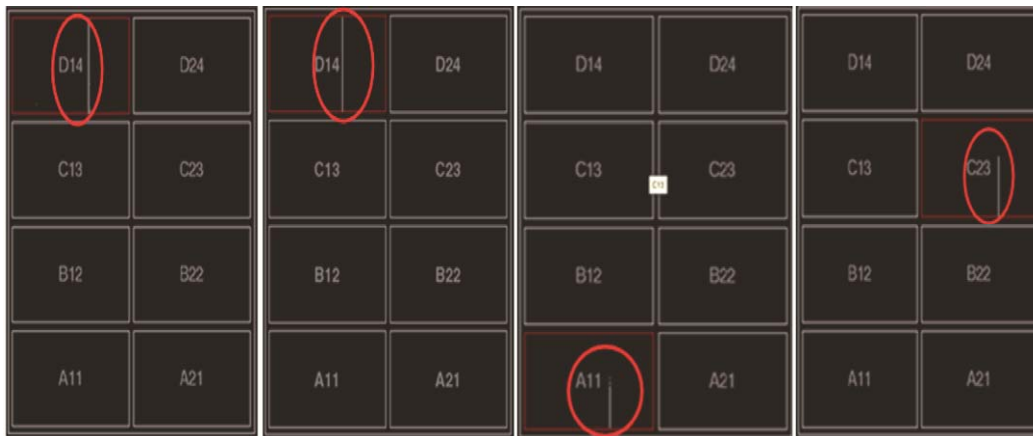
Fig. 21. The shorted area is reduced to a line or partial line.
