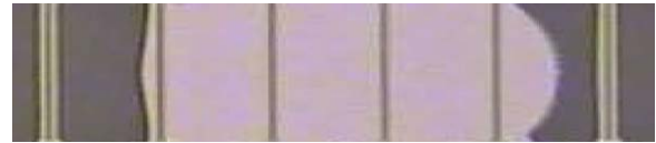
Fig. 6. Serious defect with a large area shorted.
