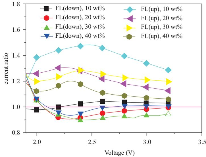
Fig. 7. The relationship between current ratio and voltage under the action of the Lozentz force. (Inter-electrode distance of 5 mm, the magnetic force of 4.5T).
