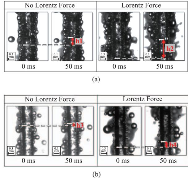
Fig. 4. The rising velocity of hydrogen gas bubbles at various current density. (a) 0.3 A/cm<sup>2</sup>, and (b) 0.1 A/cm<sup>2</sup>.
