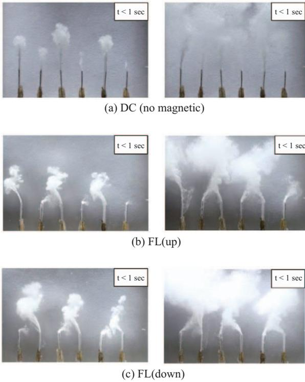
Fig. 3. The bubble motion diagrams observed in multi-electrode cell. (a) without magnetic field, (b) with upward magnetic field, (c) with downward magnetic field.
