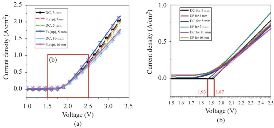
Fig. 6. The electrolytic performance of the electrode with or without FL(up) at various electrode distances. (a) the I-V curve, (b) the decomposition voltage.
