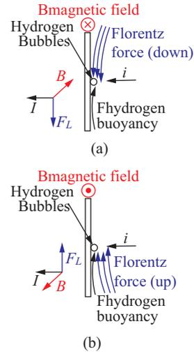
Fig. 1. The effect of the flow field near the cathode. (a) downward Lorentz force, (b) upward Lorentz force.
