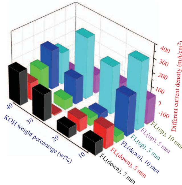
Fig. 8. A 3D diagram to show the effects of magnetic field, electrode distance and KOH concentration on the current densities.
