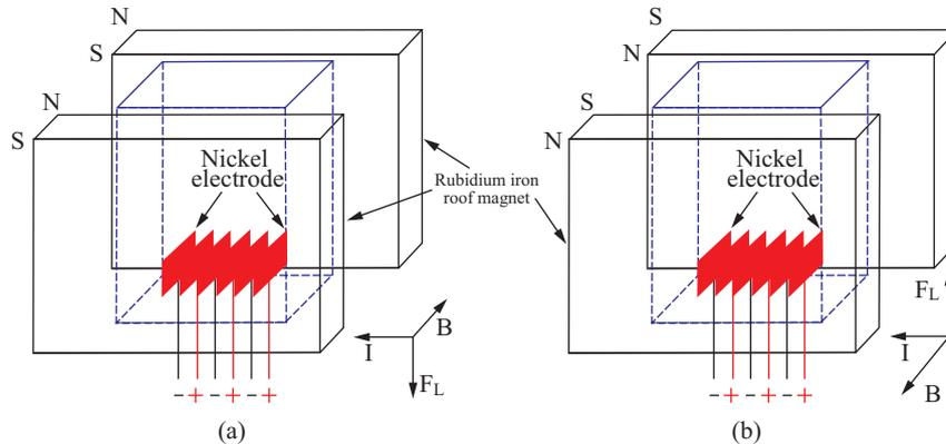
Fig. 2. The experimental set-up of the electrolytic cell. (a) downward Lorentz force, (b) upward Lorentz force.
