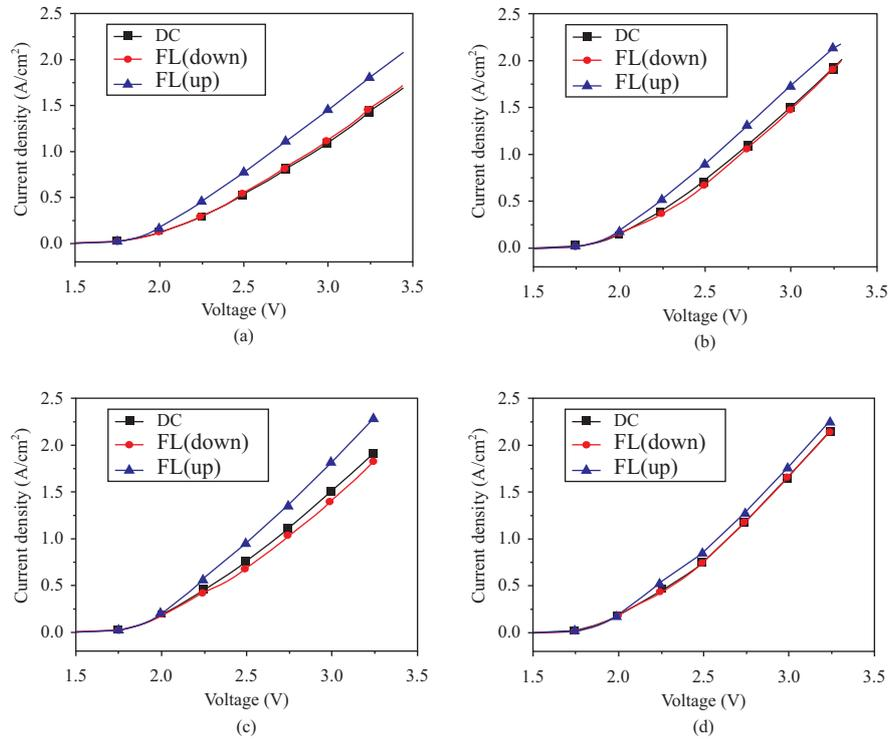
Fig. 5. The I-V curves of the electrode with the Lorentz force in various KOH electrolyte concentrations. (a) 10 wt%, (b) 20 wt%, (c) 30 wt%, (d) 40 wt%.
