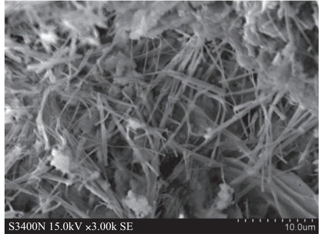
Fig. 10. SEM (3000×) image of the region 5 mm beneath the surface of PSM.
