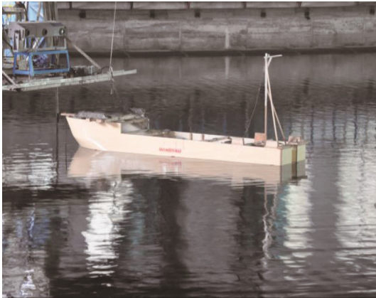
Fig. 3. Roll decay test of HYSY201 vessel model.
