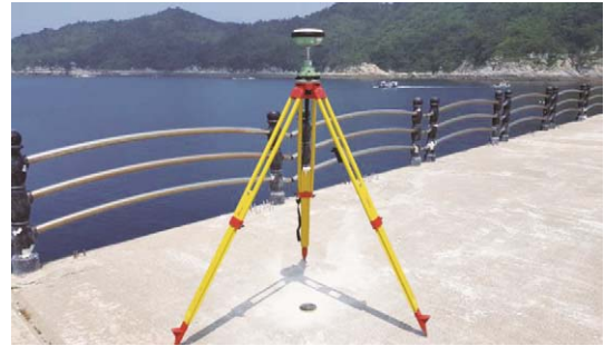
Fig. 3. GNSS observation at a datum point.
