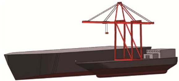
Fig. 6. Multi-body dynamics mechanical model of OCC system.
