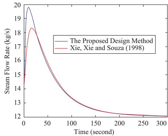
Fig. 4. Responses of steam flow rate  $y_4(t)$ .
