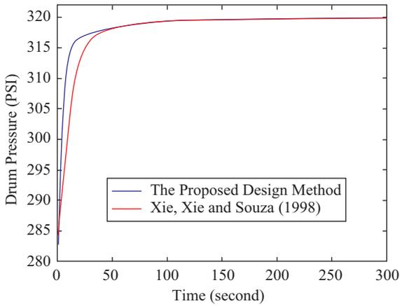
Fig. 1. Responses of measured drum pressure  $y_1(t)$ .
