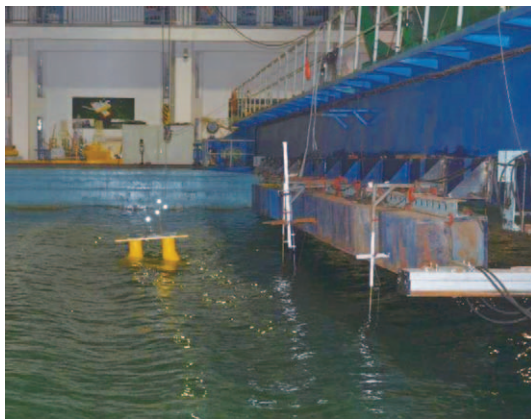
Fig. 7. Model test of FDPSO in the State Key Laboratory of Ocean Engineering.
