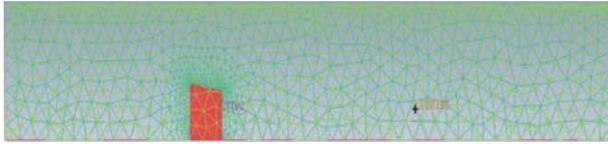
Fig. 4. Division of calculation domain with mesh.
