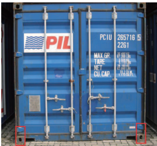
Fig. 8 The experimental results of corner casting detection.
