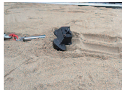
(c) Begin to insert into soil (57N)
