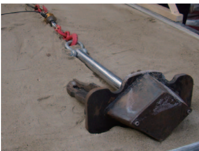
(a) Placed on soil surface (385N)
