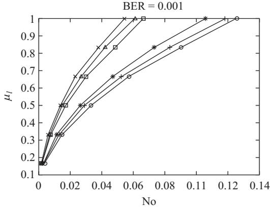
Fig. 3. Transmission power weighting of the FBMC-LDPC UTA scheme with a BER of  $10^{-3}$ , for PCE and CEEs of 5% and 10%.
