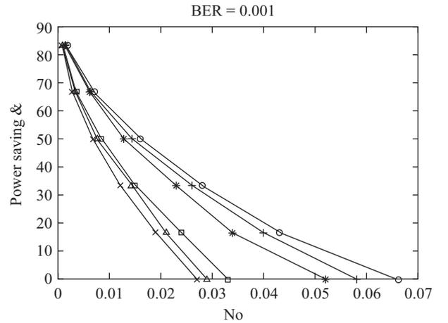
Fig. 6. Power saving ratios of the FBMC-LDPC UTA scheme with a BER of  $10^{-4}$ , for PCE and CEEs of 5% and 10%.
