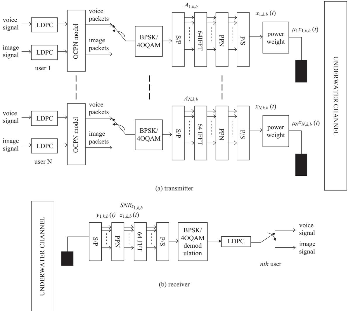
**Fig. 1. Proposed FBMC-LDPC based UTA for voice and image transmission.**
