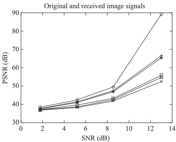
Fig. 8. PSNRs of original and received image signals with PCE and CEEs of 5% and 10%.
