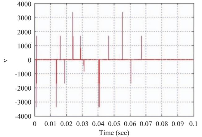
Fig. 10. Voice signal received using 4-OQAM with a CEE of 5%, BER of  $10^{-2}$ , and MSE of 18795.
