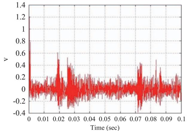
Fig. 11. Voice signal received using 4-OQAM with a CEE of 5%, BER of  $10^{-3}$ , and MSE of 0.00002984.
