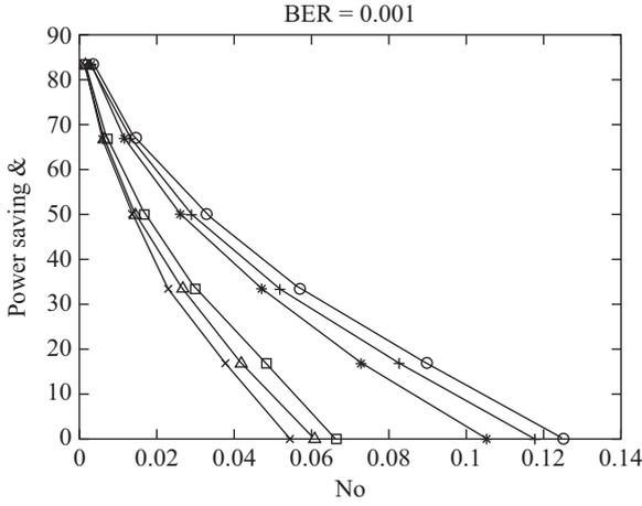
Fig. 4. Power saving ratios of the FBMC-LDPC UTA scheme with a BER of  $10^{-3}$ , for PCE and CEEs of 5% and 10%.
