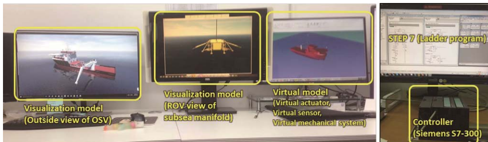
Fig. 17. Implementation of HILS in the AHC system.
