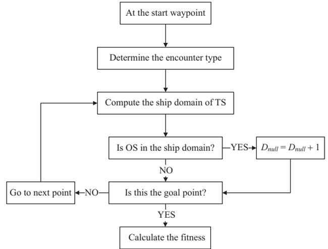
Fig. 5. Calculation process for the fitness of each particle.
