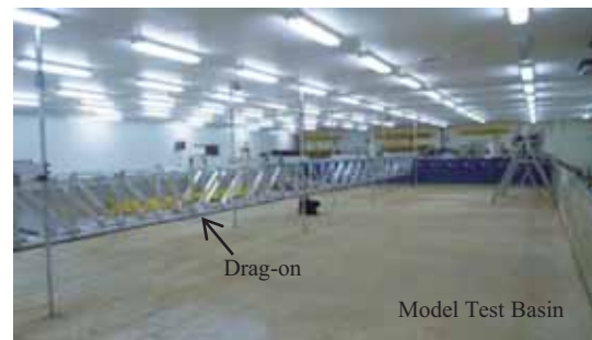
Fig. B3. Drag-on setup within empty Model Test Basin.
