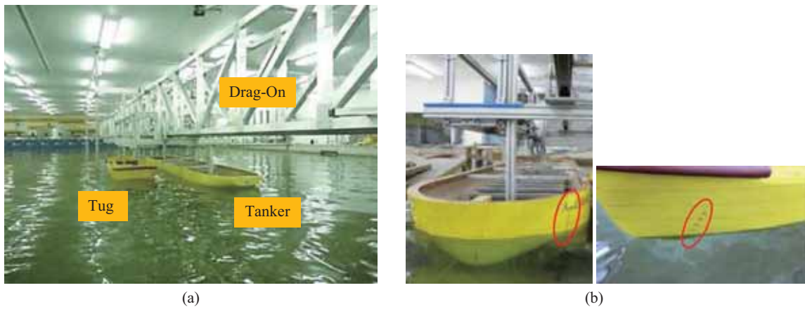
Fig. 8. (a) Experimental setup for interaction between vessels in AMC's Model Test Basin and (b) Turbulence simulators used on the models: left image wire on tanker model and right image studs on tug model.
