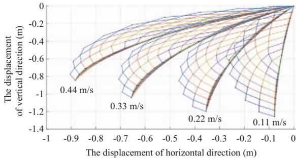
Fig. 4. Side view of profile of netting in different current with breakage.
