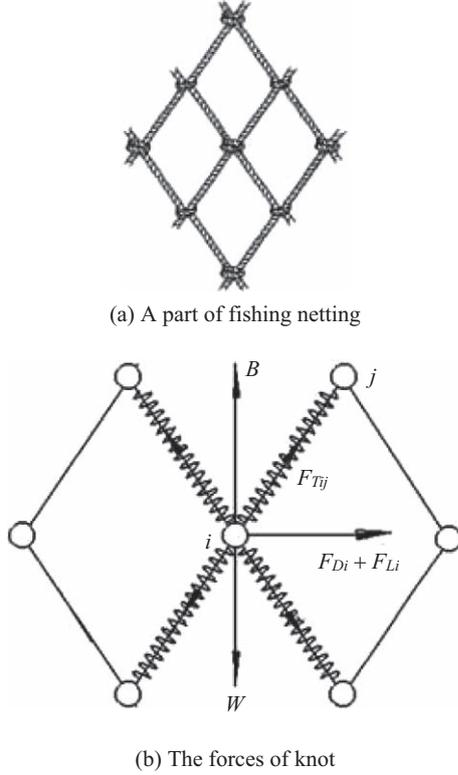
Fig. 1. Schematic diagram of the model used for the calculation for mesh knots.
