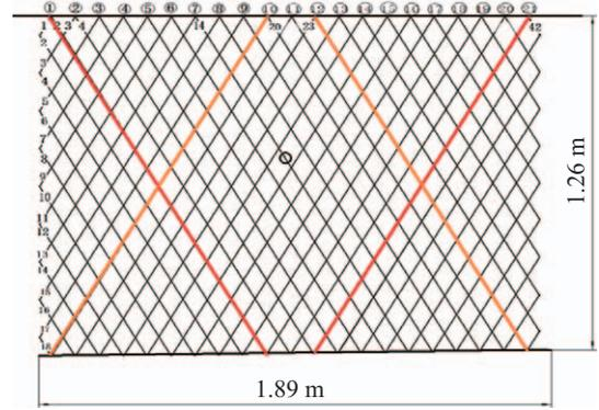
**Fig. 2. Structure of plane net.**
