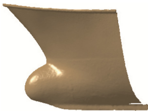
Fig. 14 Triangular mesh surface of the processed data
