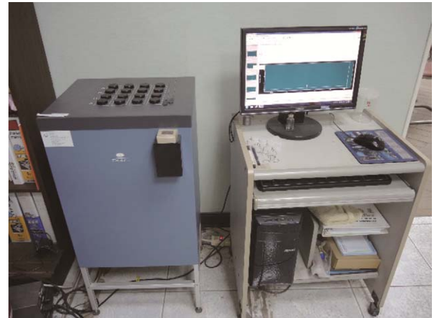
Fig. 3. Setup of an isothermal calorimeter to measure the heat of hydration.
