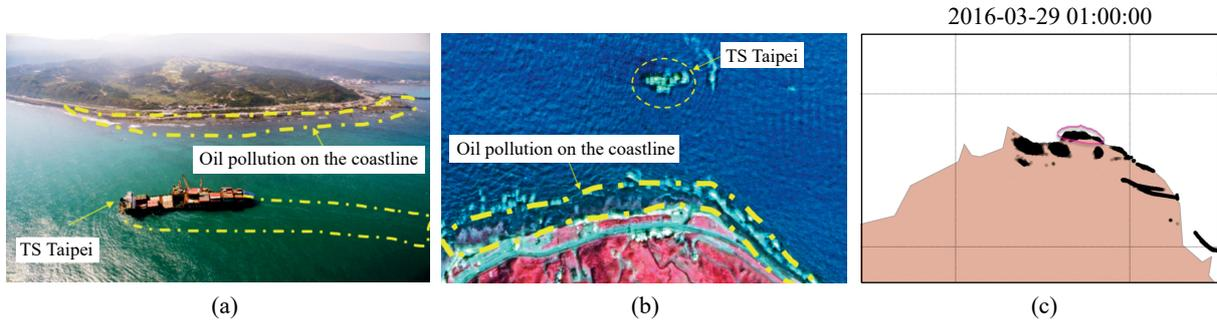
Fig. 12. Images from (a) unmanned aerial vehicles (UAVs) at 02:24 and (b) FORMOSAT 2 at 02:03 compared to (c) the simulation results at 01:00 on March 29, 2016.
