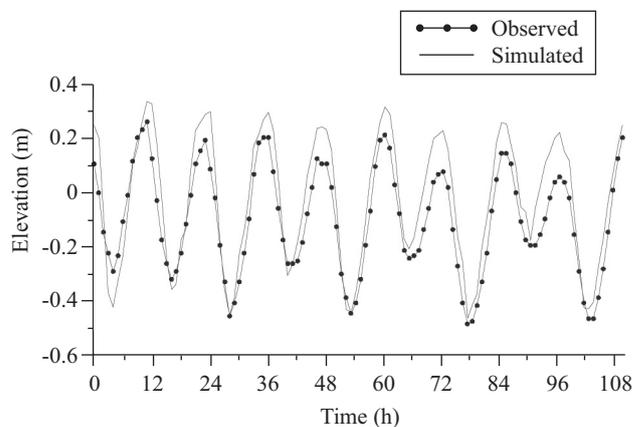
**Fig. 7. Comparison of the elevation taken simulations and observations at Keelung Station.**
