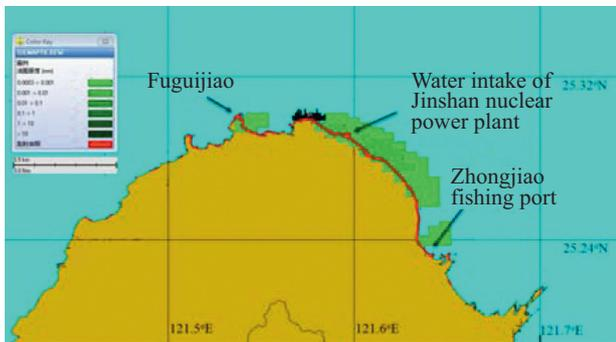
Fig. 13. The results of the OILMAP simulation at 10:00 on March 27.
