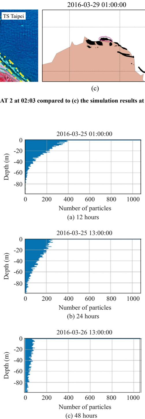
Fig. 15. Vertical distribution of oil droplets simulated in the water column after (a) 12 hours, (b) 24 hours, and (c) 48 hours.
