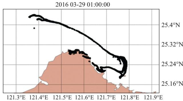
Fig. 9. Simulation results at 01:00 on March 29 (108 hours after the oil spill).
