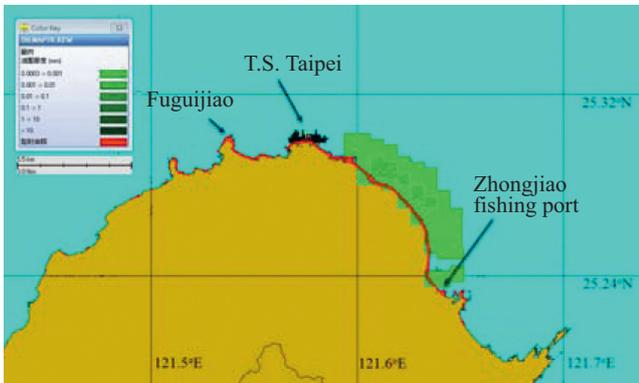
Fig. 14. The results of the OILMAP simulation at 02:00 on March 28.
