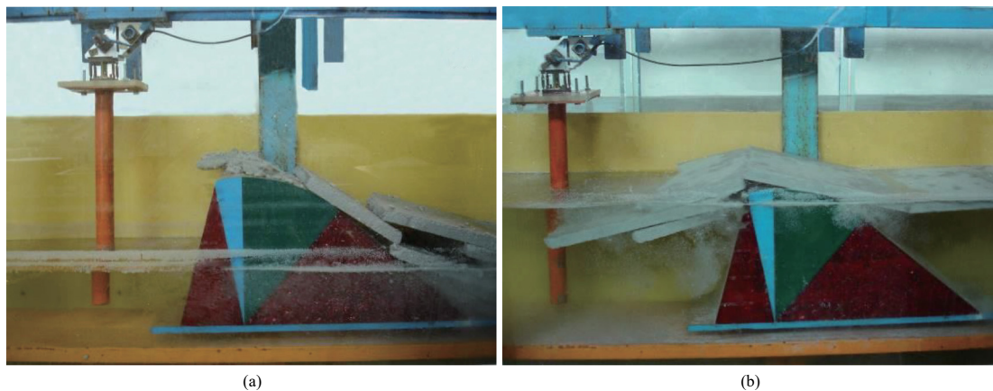
Fig. 3. Ice failure on the IBS at different water levels. Pile-up occurs upstream at the low water level (a). Ice ride-up on the IBS and its impact on the ICP at the high water level (b).
