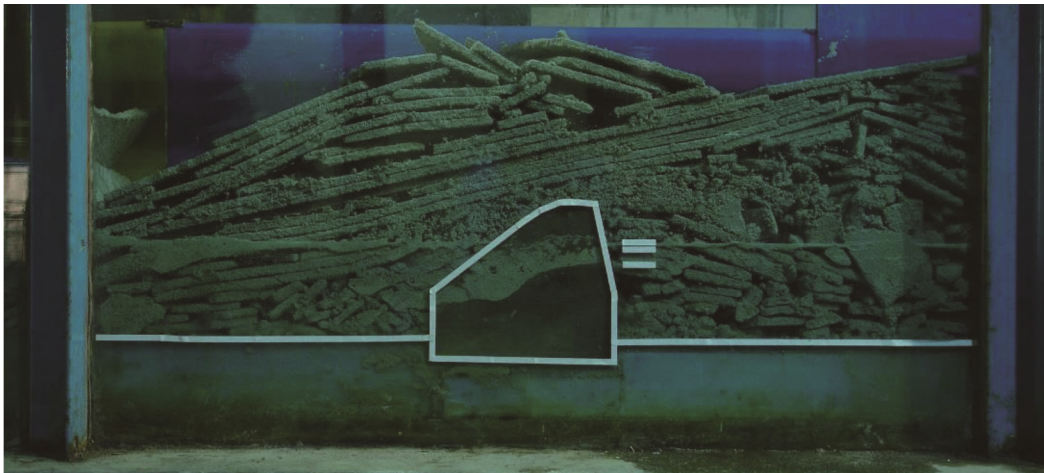
Fig. 12. A new rubble on the sloping surface of the original rubble.
