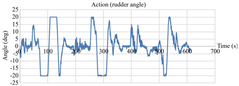
Fig. 23. Rudder angle of the autonomous ship as a function of time in Case 3-1.
