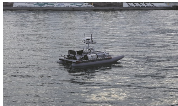
Fig. 15. USV during DP performance test
