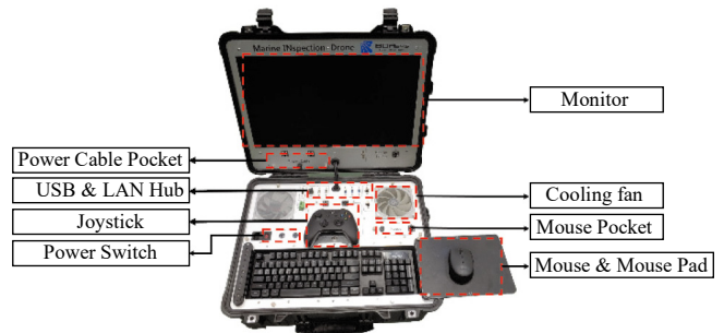
Fig. 5. Configuration of operation console
