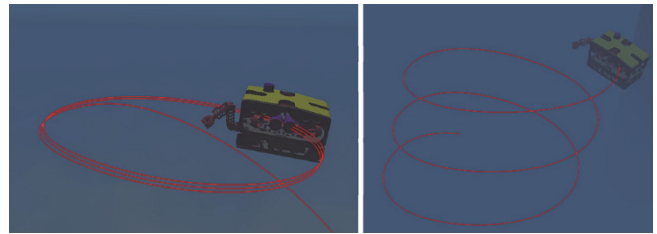
Fig. 10. Turning circle and helix trajectory of the ROV driven by the user.
