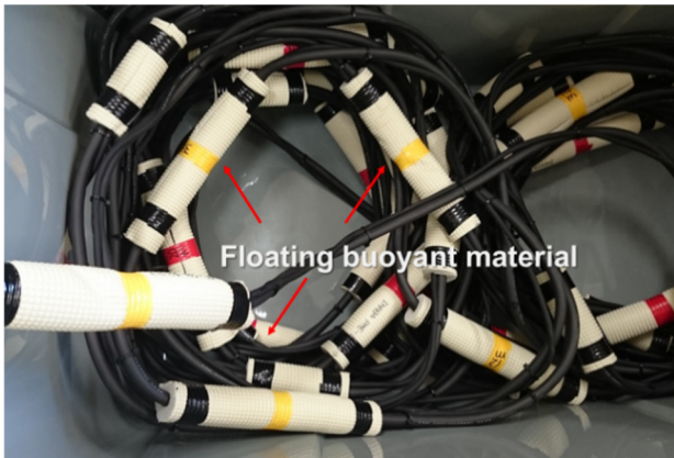
Fig. 5. Umbilical cable and floats
