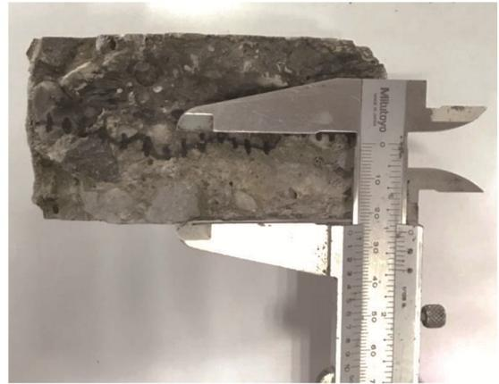
Fig. 2. Illustration of measurement for chloride penetration depth
